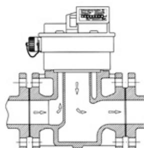
Operative measuring point with gas meter with over-run brake:
