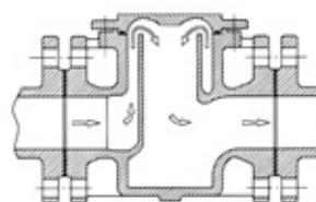
Operative measuring point with gas meter without over-run brake:
