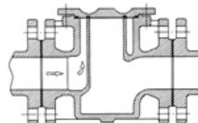
Prepared measuring point with overflow cap:
